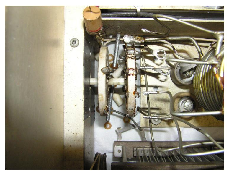
With C151 and C153 removed the switch wafers have enough clearance to slide off the shaft.
