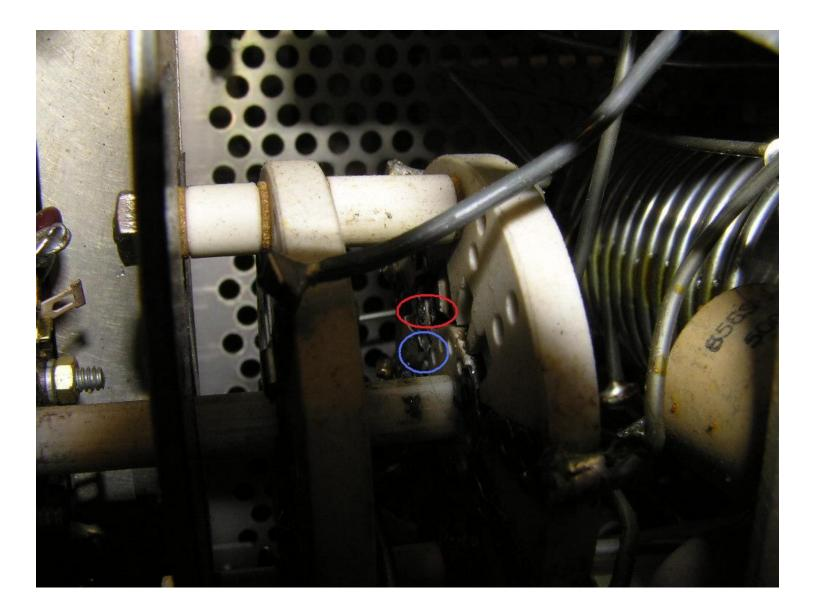
I removed C151 and C153 then de-soldered the switch and removed wires.
