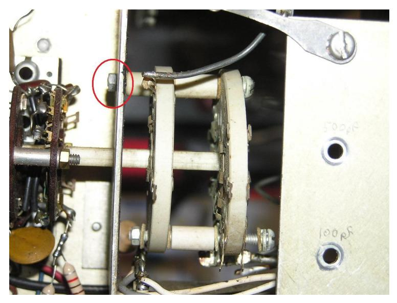
After stabilizing the top mount it is a simple matter to install the bottom spacer washers and nut. This nut is tightened to spec. at this time. Then the top nut is removed and the flat and lock washer is installed and the nut is replaced.
