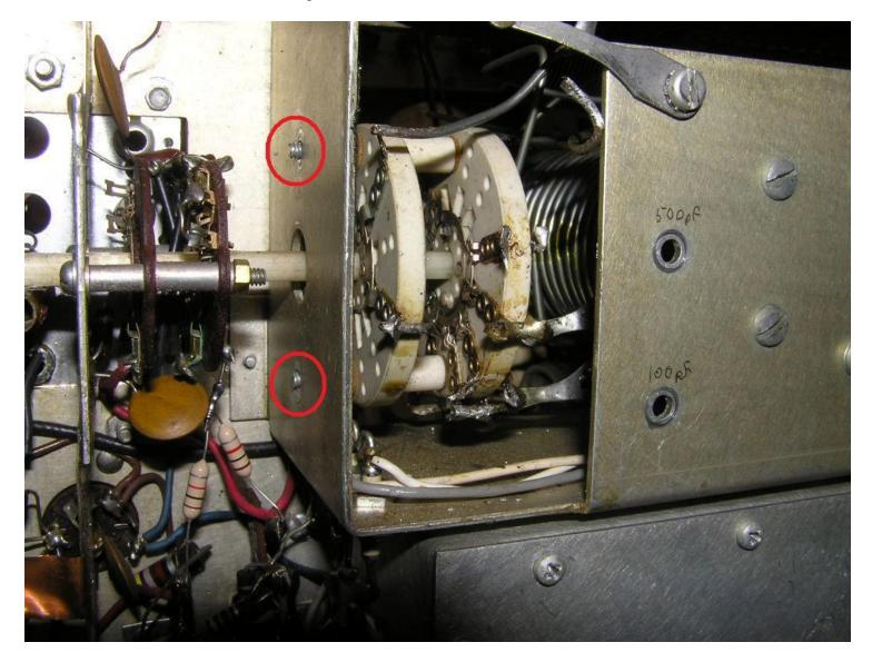
Then remove the mounting screws and let the washers and spacers fall on the dish towel under the rig.
