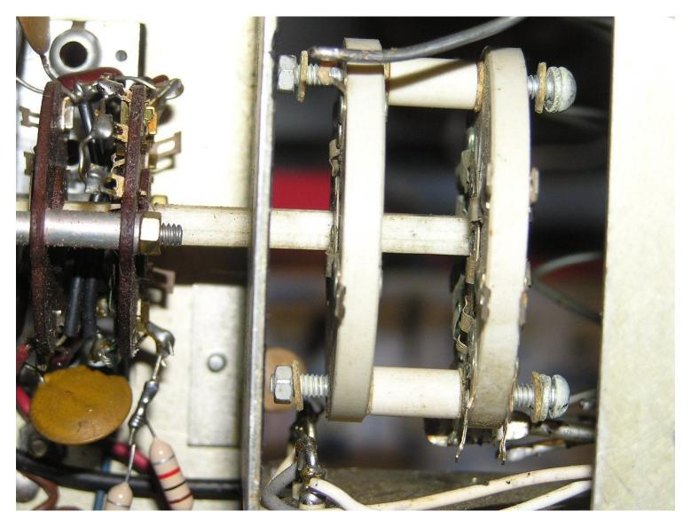
The whole assembly is rather unstable so when I installed the chassis spacer on the top side I did not try to put the flat and lock washer under the nut at this time. The nut is lightly snugged just enough to stabilize the assembly
