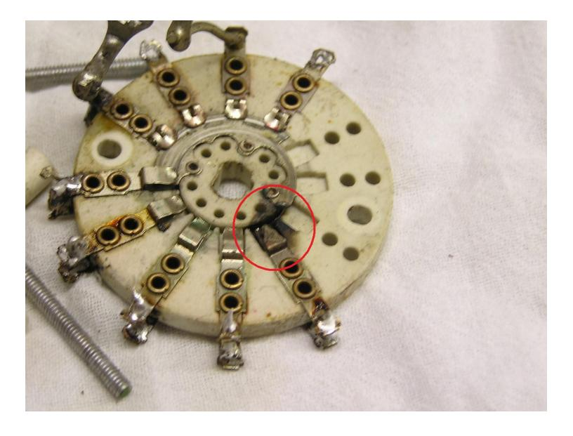
Next loosely assemble and preset rotor portion of each switch.
